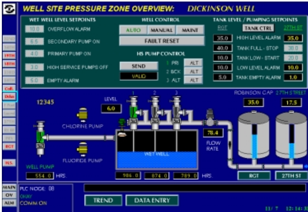
Figure 5. SCADA screen showing status of a well site
